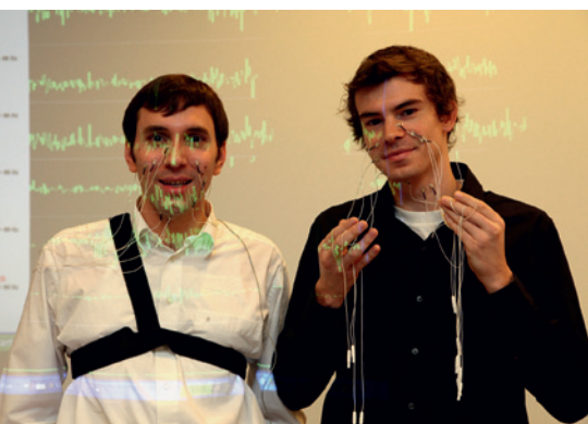
Electrodes capture the electromyographic signal at the surface of the facial skin
